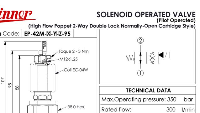
Cavity-Tooling: 42M-2 Installation torque: 110 - 130 Nm
